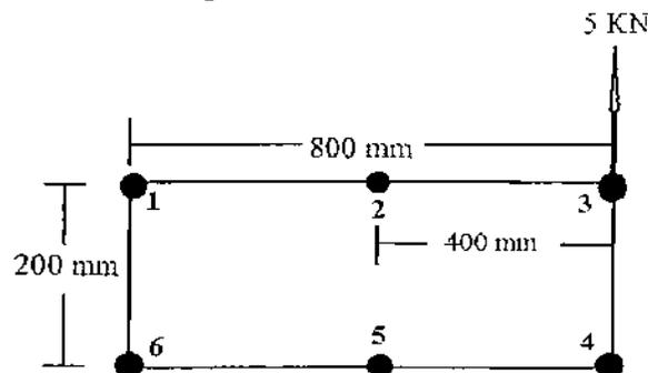
7- The figure below shows a three cell thin wall wing box made from a material whose shear modulus  $G$  is 18 GPa. The wing box is subjected to a constant clockwise torque of 12,000 N.m. The upper panels of the box have a constant thickness of 2.5 mm, while the lower panels have a thickness of 1.75 mm. All vertical panels are 1.5 mm in thickness.
