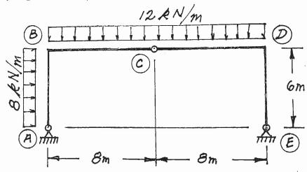
Use the principle of virtual work to calculate the vertical deflection at point  $\bigcirc$  on beam  $\bigcirc$  -  $\bigcirc$  of the structure shown. The beam is inextensible and has  $EI = 5.0 \times 10^4 \text{ kN.m}^2$ . The tie rod does not take moment and has an AE = 5200 kN.
