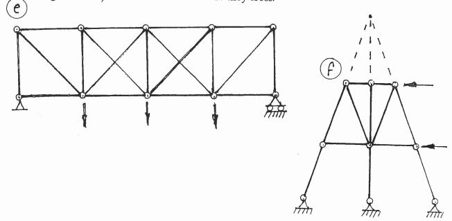
(18) 2. For each structure shown, compute the reactions and draw shear and bending moment diagrams. Indicate which are positive and which are negative segments of each bending moment diagram. For each shear and bending moment diagram, calculate and indicate the magnitudes of the maximum positive and negative ordinates.
