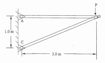
2. Determine the magnitude and direction (up or down) of the force P if the displacement at A is not to exceed 2 mm (down). Take E = 200 GPa and  $I = 750 \times 10^6$  mm<sup>4</sup>.
