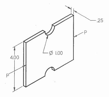
A notched T6 aluminum alloy is show above. All dimensions are in inches. An axial load, *P*, of 400 kN is applied to each end.
