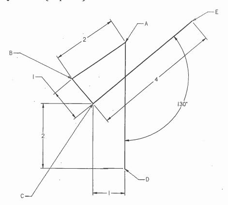
The above diagram is schematic of a small manual press or juicer. Points C and D are grounded. Link AD has variable length. Link AB is fixed length. Link BCE is rigid with a right angle between lines BC and CE. The dimensions are in inches. The user exerts a force up at E causing A to be become displaced down for the given position of 130 degrees. For this position, determine the following.
