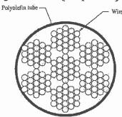
The above schematics shows the cross-section of a cable manufactured from 7×19 braided carbon steel wire. The cable is subjected to twisting and bending that opens and closes the cable wire bundles during operation. The operating environment contains both moisture and salt.
