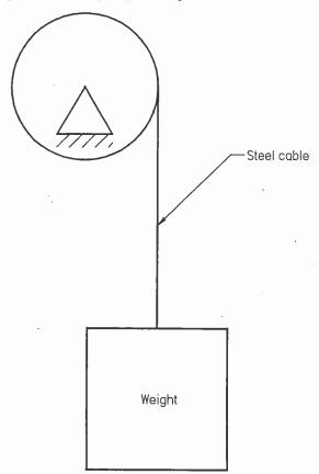
Select a stranded steel cable for the above schematic. The cable must be able to withstand the sudden stop, from 10 m per minute, of the 1 ton weight.
