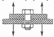
Two grade 252 cast-iron components, carrying a static load of 10 kN and each 20 mm thick, are held together by four bolts. The components are not intended to be separated again once built.
